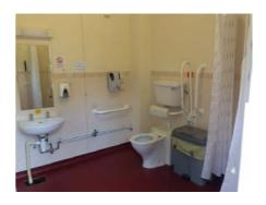
The **male and female toilets** have inward-opening doors with clear openings of 800mm. There is a 170mm step up into a lobby. The lobby has an outward-opening door with a 700mm clear opening. Both doors are stiff to open. In both male and female toilets, one shower cubicle, one privacy cubicle and one WC cubicle are fitted with grab rails. The taps to the washbasins are lever non-mixer. The accessible WC/shower is used instead.
